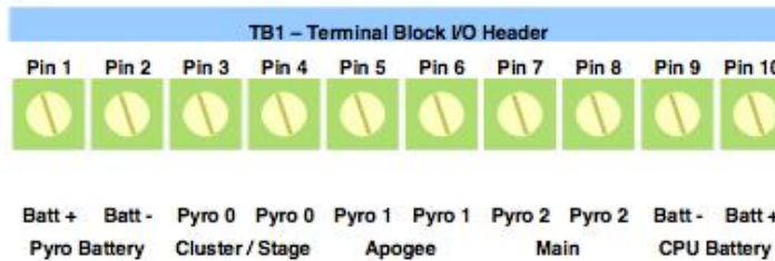
Fig. 2. G-Whiz altimeter/accelerometer used for altitude and speed verification as well as a backup for controlling parachute ejection charges.
